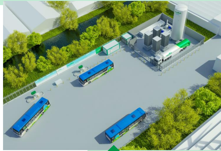
Liquid based Station (350 bar) Up to 5 tons/day Buses Large Fleets
